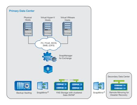
Figure 1) SnapManager in a Fibre Channel or iSCSI environment.
